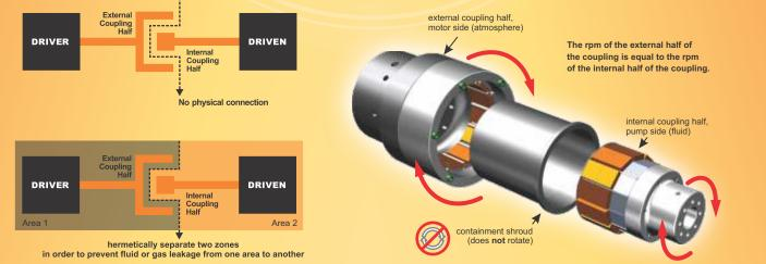
Magnetic couplings capable of transmitting torque from 3 to 600 Nm without mechanical contact between two shafts through magnetic forces that are established between the internal and external rotor. The magnetic coupling is ideal for applications where prevention of leakage from the pump is essential. Magnetic couplings also prevent vibrations and, radial and axial loads to the pump shaft. The magnetic coupling is a synchronous system with a primary function of hermetically separating two areas.
