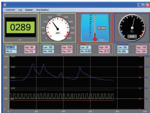
Left. The real time display showing the range of display options that can be set up for each of the four channels
